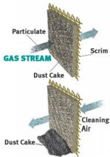
Non-membrane filter lets dust get inside filter media reducing cleanability and increasing pressure drop.
