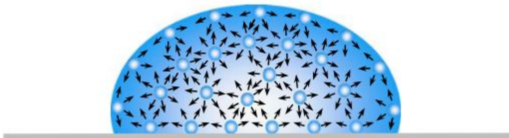
Fig. 2. Surface tension is caused by the unbalanced forces of liquid molecules at the surface [3].
